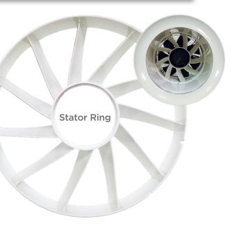
ZOO Fans' proprietary stator ring reduces centrifugal and angular flow, straightens the air column, boost air speed, and significantly increases throw.
