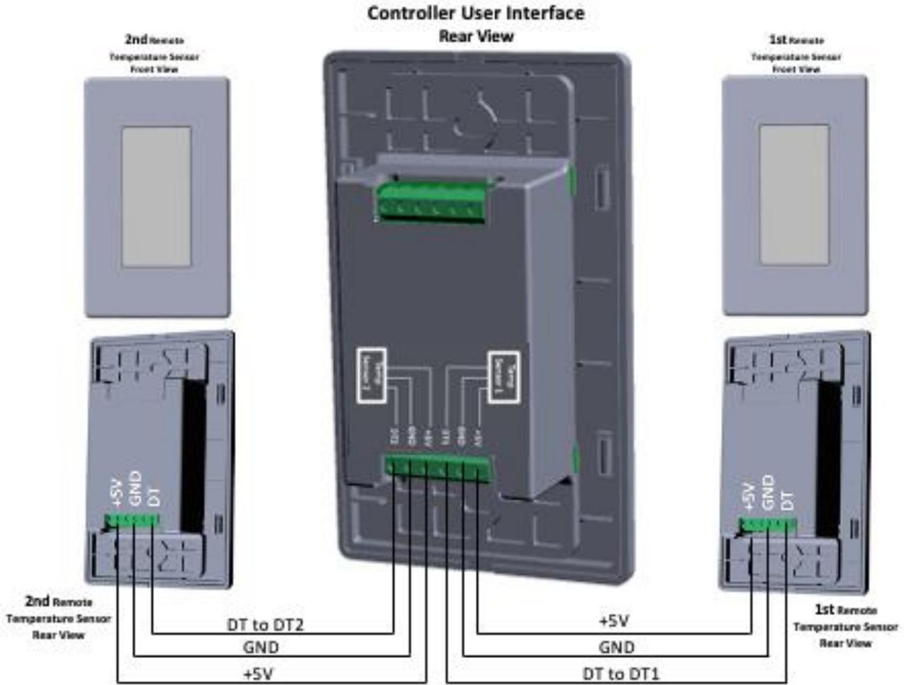
For vertical destratification, install one temperature sensor near the ceiling approximately 18" from roof deck and another near the floor (within 12" if possible). To equalize temperatures horizontally, install one temperature sensor in each area. The controller will constantly calculate the difference in temperature between the two sensors and adjust the fan speed higher and lower as required to maintain equalization of temperatures.
