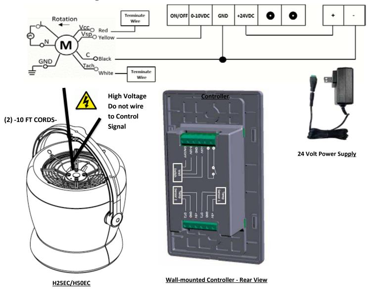
Electrical connection should be made according to the wiring diagram. Wires should be terminated using the horizontal terminal blocks (included). Shielded cable is recommended to reduce interference. Use Stranded Wire. DO NOT use solid wire
