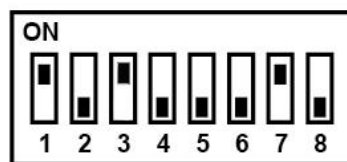
BMS LOSS OF SIGNAL: OFF
